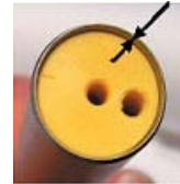
Figure 1: Average tube wall thickness 0.035"/0.889 mm
